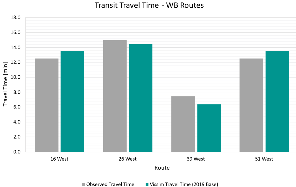
Figure 9: Model Validation – Modelled vs Observed Westbound Bus Routes (on McKenzie)
